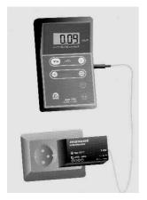
The DGM-1500 has a connector for a mains adapter, allowing it to be used for round-the-clock radiation monitoring. A wall mounting bracket for the meter is available as an optional extra, so the meter can be installed where it is always easily visible. The alarm level is userprogrammable. If the level of the measured radiation exceeds the alarm level a warning tone is emitted (see the section on programming the alarm level).
